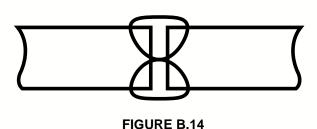
In the example shown in Figure B.14, the joint has been welded so that 100% penetration could be achieved. The weld, if properly made, is as strong as or stronger than the original metal.
